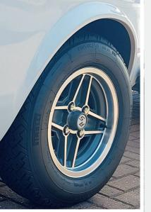
is to stop the bead slipping into the wheel well under cornering forces. At Longstone Tyres we suggest that if it doesn't have that safety hump, fit an inner tube. If you are dubious about whether your wheel is designed to run tubeless, or an alloy wheel that has become porous, simply fit an inner tube. We sell the Michelin inner tubes because the quality is exceptional. Do not fit inner tubes in tyres lower than a 70 profile.
